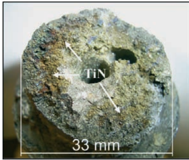
Fig. 7. Formation of TiN in aluminothermic TiAl at the broken electrode surface using a copper mould (electrode head).
