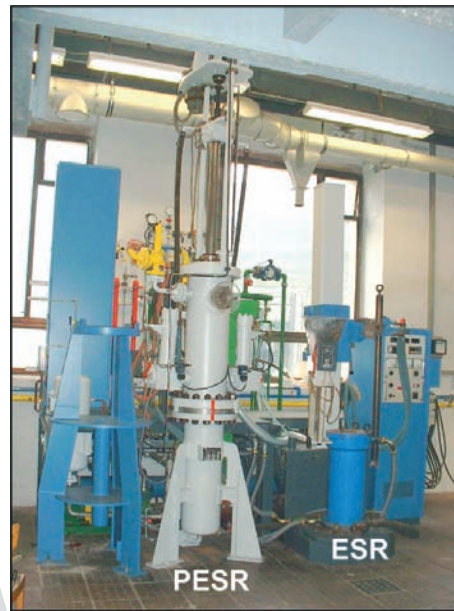
Figure 10. PESR/ESR pilot scale furnace at IME Aachen.
