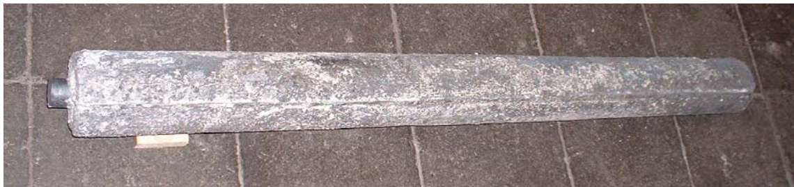
Figure 2: ATR-cast TiAlX electrode ( \varnothing 110 mm, L 1350 mm, approx. 60 kg) for ESR refining
