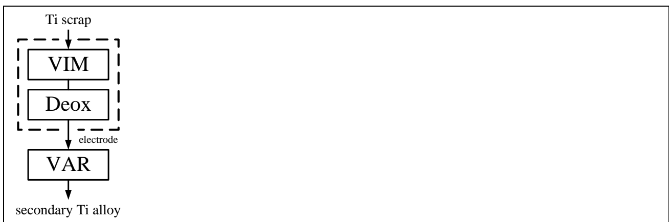
Figure 1: simplified process steps of the recycling concept at IME
