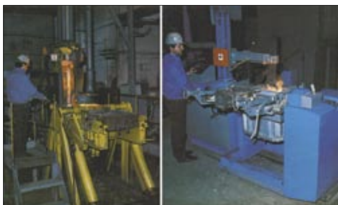
Fig. 8: Stationary a) and portable b) versions of ESCR furnaces
